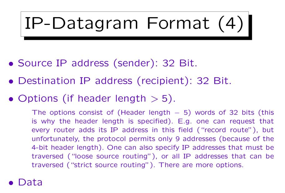
Length of Data in bytes = Total length - Header length \* 4.
