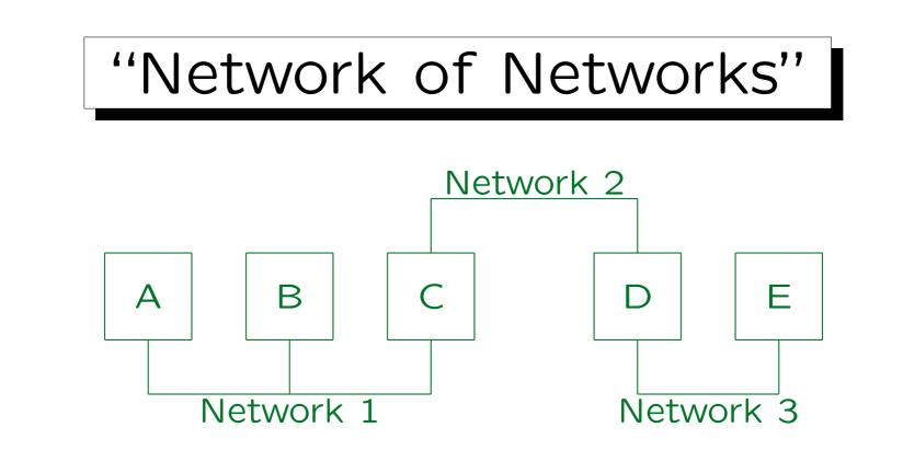
If machine A wants to send data to machine E, the data packages must be relayed via machines C and D.
