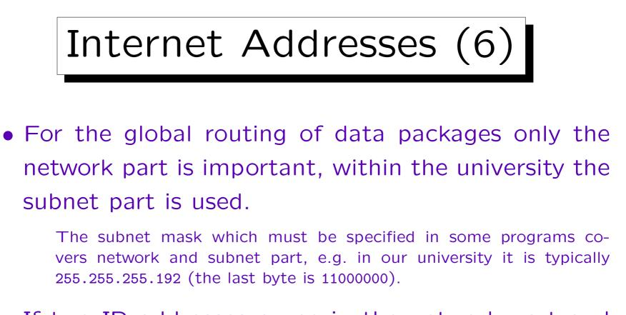
If two IP addresses agree in the network part and in the subnet part, the computers are connected to the same network.
