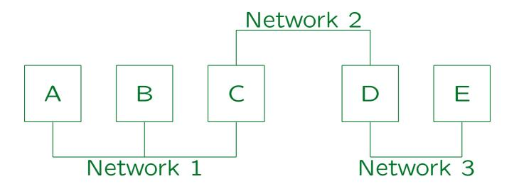
If machine A wants to send data to machine E, the data packages must be relayed via machines C and D.
