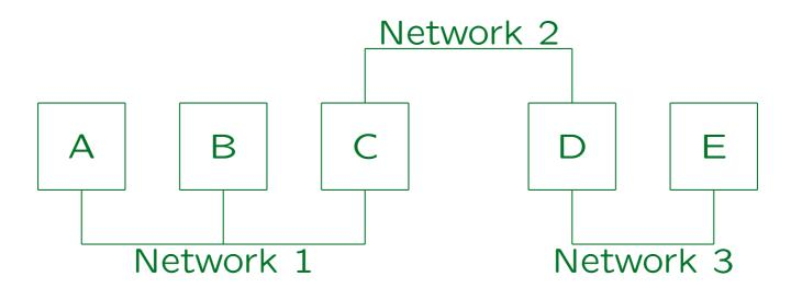
If machine A wants to send data to machine E, the data packages must be relayed via machines C and D.
