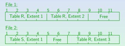
Tables R and S are stored in a tablespace which consists of two data files. Table R has three extents: Block 1 to 4 in File 1, Block 5 to 8 in File 1, and Block 7 to 11 in File 2. Oracle does not merge contiguous extents of a table. Table S consists of a single extent (Block 1 to 4 in File 2).
