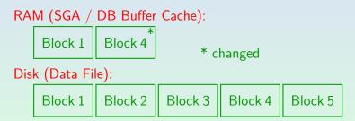
Accesses to RAM are much faster than accesses to disk, but the RAM is usually smaller (and volatile).
