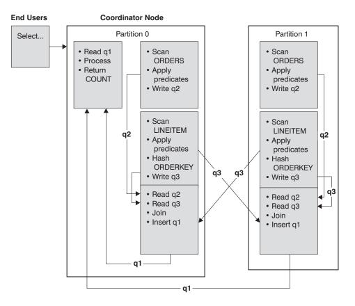
The ORDERS table is partitioned on the ORDERKEY column. The LINEITEM table is partitioned on a different column. The LINEITEM table is hashed and sent to the correct ORDERS table database partition. In this example, the join predicate is assumed to be: ORDERS.ORDERKEY = LINEITEM.ORDERKEY.
