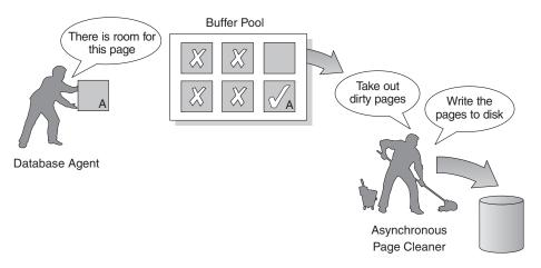
Figure 23. Asynchronous page cleaner. "Dirty" pages are written out to disk.
