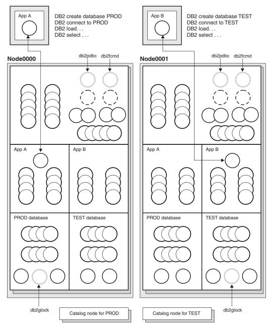
Figure 10. Process model and multiple partitions
