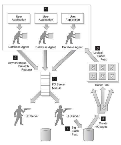
Figure 24. Prefetching data using I/O servers
