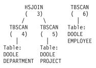
The first part of the plan accesses the DEPARTMENT and PROJECT tables and uses a hash join to join them. The result of this join is joined to the EMPLOYEE table. The resulting rows are returned to the application.
