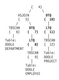
This plan is similar to that in the third example, except that multiple subagents execute each subsection. Also, at the end of each subsection, a local table queue gathers the results from all of the subagents before the qualifying rows are inserted into the second table queue to be hashed to a specific node.
