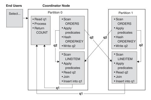
The LINEITEM table is partitioned on the ORDERKEY column. The ORDERS table is partitioned on a different column. The ORDERS table is hashed and sent to the correct LINEITEM table database partition. In this example, the join predicate is assumed to be: ORDERS.ORDERKEY = LINEITEM.ORDERKEY.
