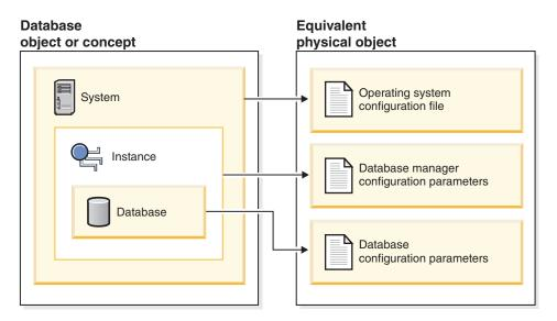
Figure 33. Relationship between database objects and configuration files
