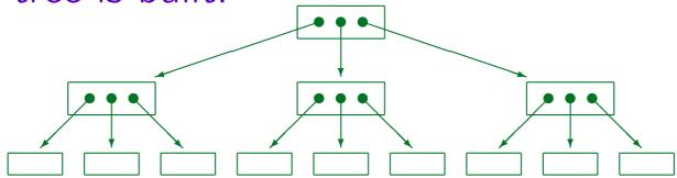
• The blocks in the lowest level ("leaf blocks") contain all occurring customer numbers (in ordered sequence) together with the address ("ROWID") of the corresponding CUSTOMERS row.
